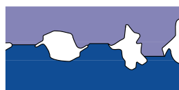
If the surfaces are smooth the contact points are modest and provide high slippage
