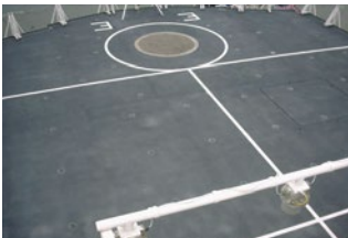
Flight deck – Completed with white markings
